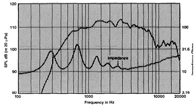
Frequency response of the 2446J coupled to a JBL 2380A Flat-Front Bi-Radial® Horn, measured on-axis at a distance of 1 meter with a 1-watt (4.0 V rms) input in a reflection-free environment, with impedance vs. frequency curve. A horn with a pure exponential flare, such as typical radial horn designs, will exhibit greater high-frequency output on-axis at the expense of lose angular coverage.
