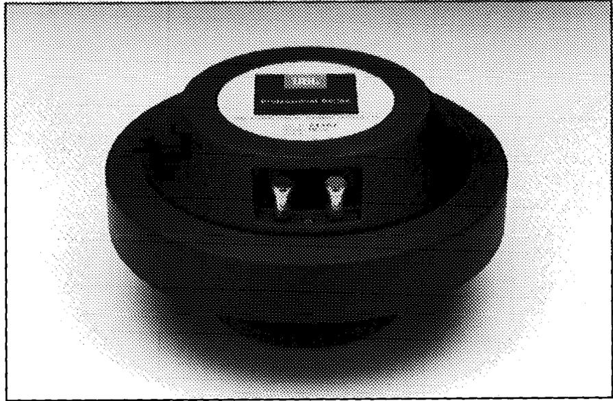
The model 2446H/J is a professional quality high-frequency compression driver that incorporates JBL's newly-developed Coherent Wave phasing plug as well as a pure titanium diaphragm with radial ribs and patented three-dimensional diamond pattern suspension.
