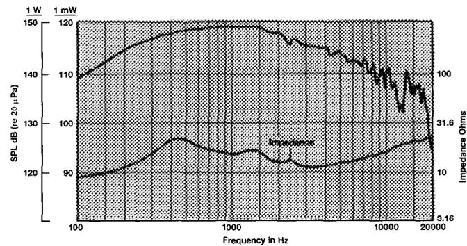
Frequency response and impedance modulus of Model 2446J coupled to as 49 mm (2 in) tube, with sensitivity referred to a 25 mm (1 in) tube. This is the power response of the transducer, and is the frequency response that will be obtained on a true full-range constant directivity horn design, such as JBL's 2360 series of constant coverage Bi-Radial® horns.
