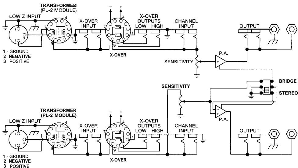
each crossover having a balanced input (11), dual (parallel) unbalanced inputs (13), an unbalanced low output (15), and an unbalanced high output (16). In order to complete the system, external patching must be accomplished between the low and high crossover outputs and the various power amp inputs using shielded patch cords. A patch diagram showing this arrangement is included at the end of this manual.
